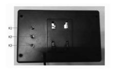
**K1:** In Menu Mode use K1 as UP function, when not in Menu Mode K1 will Turn on/off Scale Lines.
